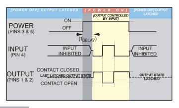
**Optional INITIAL POWER-UP DELAY (-DT option):** Upon initial power-up, the output contact remains latched and the input is temporarily inhibited during the power-up delay period (t<sub>DELAY</sub>) preventing any change in the output contact state during power-up. Power-up Delay times are available from 0.25 seconds to 60 seconds.
